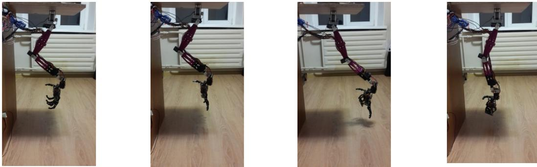
**Figure 6.** Inverse kinematics tests of a human-like manipulator prototype. It is a lightweight manipulator of 1.1 kg, it has a range of 85 cm in the workspace and a maximal payload of 0.2 kg. The length of the robot in the stretching state is 1.04 m
