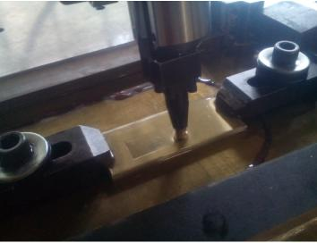
**Figure 3.** Hydrostatic tool HG6-9\_SL (K) from Ecoroll
